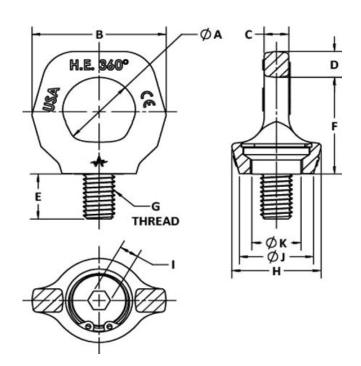
An installation key is provided to allow firm tightening by hand, which is allowable for one-time temporary lifting. For permanent installation, tighten by hex wrench to the installation torque listed in the tables below.
