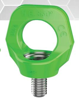
Hoist Eye 360° is a forged lifting eye that can be rotated 360° after installation, to align with pulling-force direction. This compact assembly features a specially designed shoulder bolt, which rotates freely in the precisely machined forged lifting-eye body and is held captive by a retaining ring.
